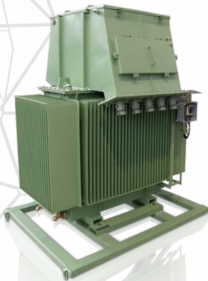
SHOCK & VIBRATION RESISTANT TRANSFORMER Type: TBN1000-12/I ; Germany Rated power: 1000kVA Rated voltage: 6000/400V
