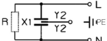
$R = 470 \text{ k}\Omega \div 2,7 \text{ M}\Omega$  on request
