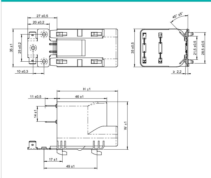
Casing: thermoplastic can, sealed with synthetical resin, flame retardant
