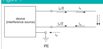
Symmetrical interference current runs in different directions in the phase and neutral conductors.
