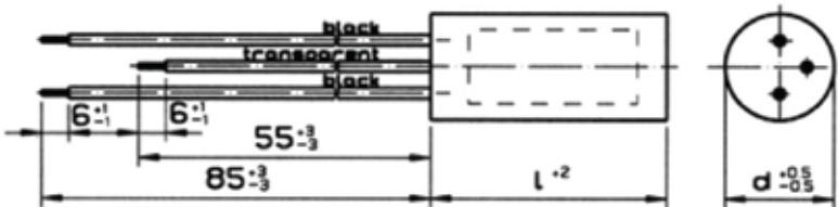
Casing: thermoplastic, sealed with synthetical resin, flame retardant.
