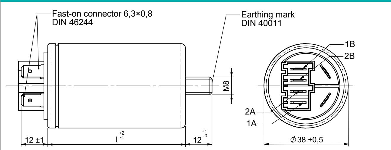
Casing: aluminium can, closed with sealing washer
