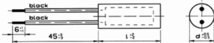
Casing: thermoplastic, sealed with synthetical resin, flame retardant
