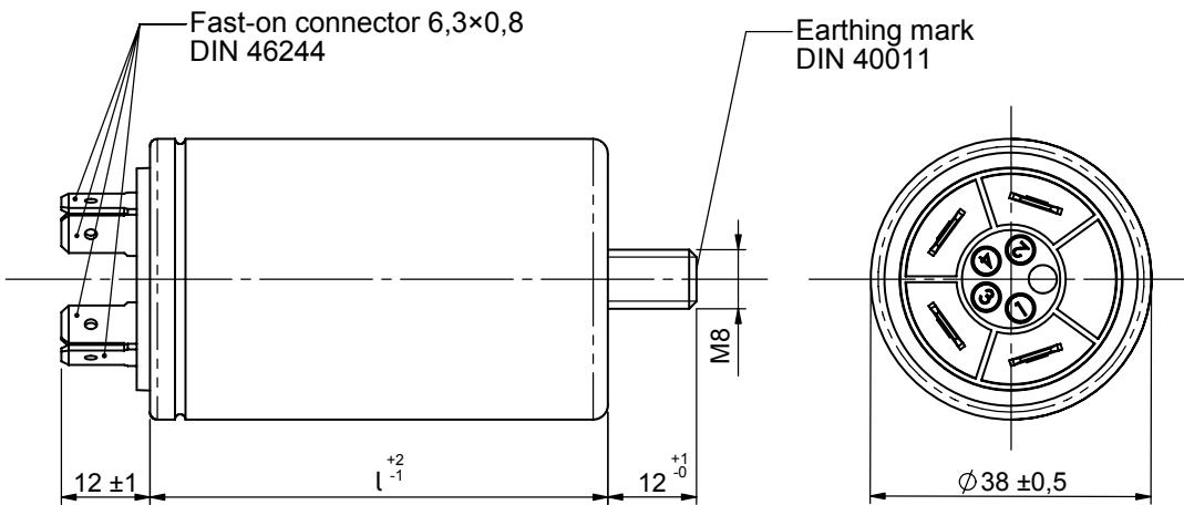
Casing: aluminium can, closed with sealing washer.
