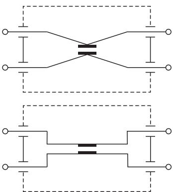
Figure 5a: single by-pass capacitor
