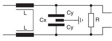
$R = 470 \text{ k}\Omega \div 2,7 \text{ M}\Omega$  on request
