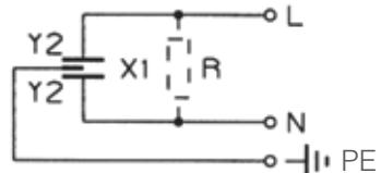
$R = 470 \text{ k}\Omega \div 2,7 \text{ M}\Omega$  on request
