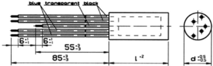
Casing: thermoplastic, sealed with synthetical resin, flame retardant.
