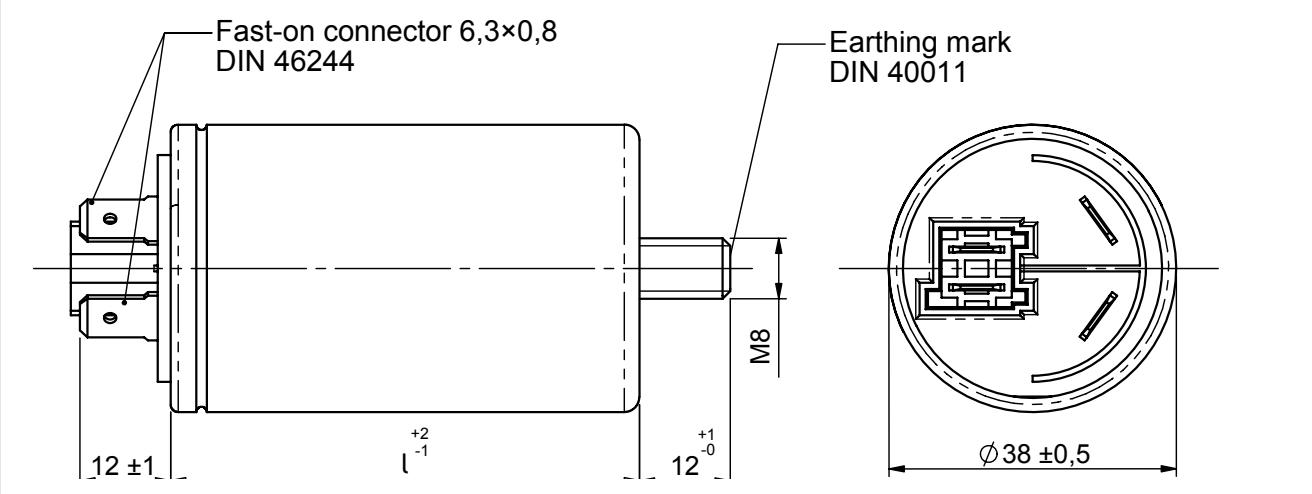
Casing: aluminium can, closed with sealing washer
