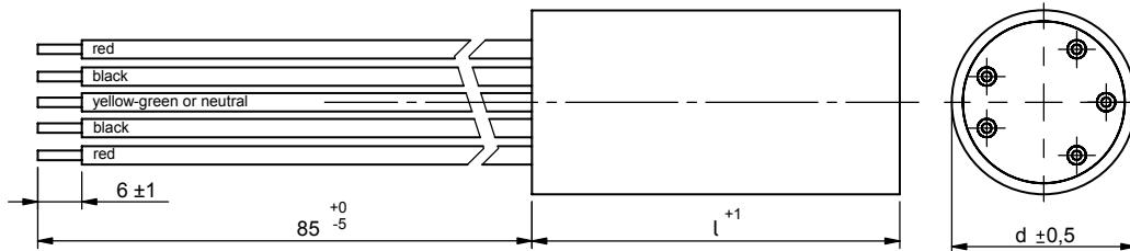
Casing: thermoplastic, sealed with synthetical resin.
