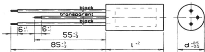
Casing: thermoplastic, sealed with synthetical resin, flame retardant
