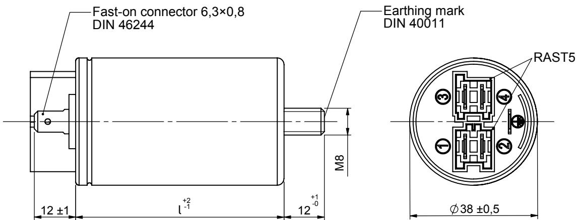
Casing: aluminium can, closed with sealing washer
