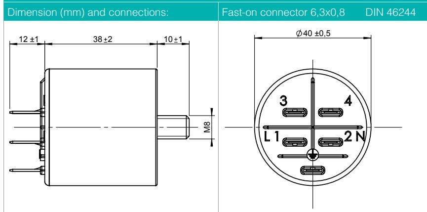
Casing: thermoplastic can, closed with sealing washer
