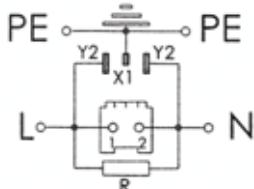
$R = 470 \text{ k}\Omega \div 2,7 \text{ M}\Omega$  on request
