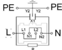
$R = 470 \text{ k}\Omega \div 2,7 \text{ M}\Omega$  on request
