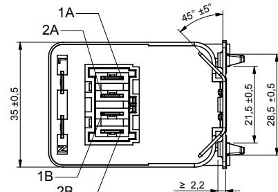
Casing: thermoplastic can, sealed with synthetical resin, flame retardant
