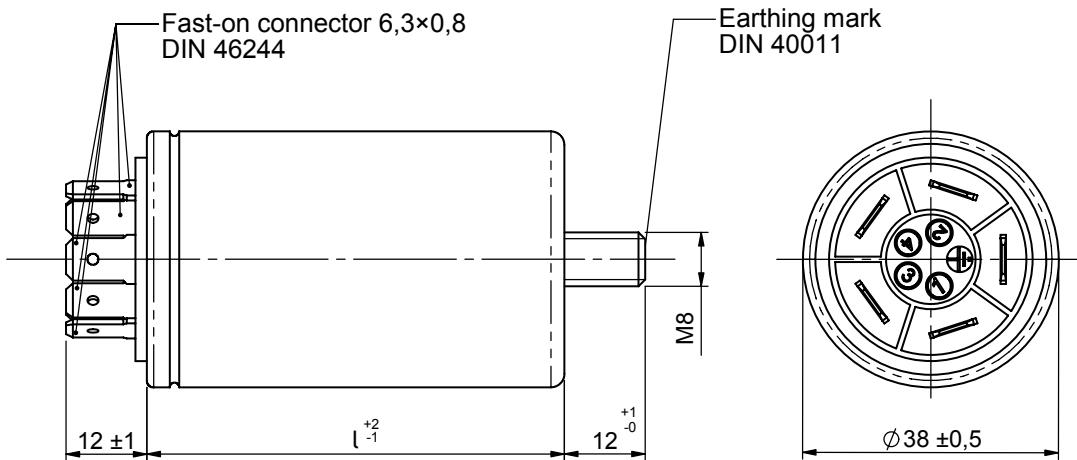
Casing: aluminium can, closed with sealing washer
