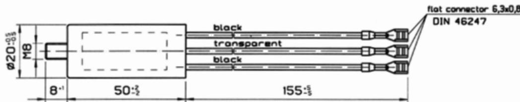
Type KPB7312 - thermoplastic can sealed with synthetical resin, flame retardant.
