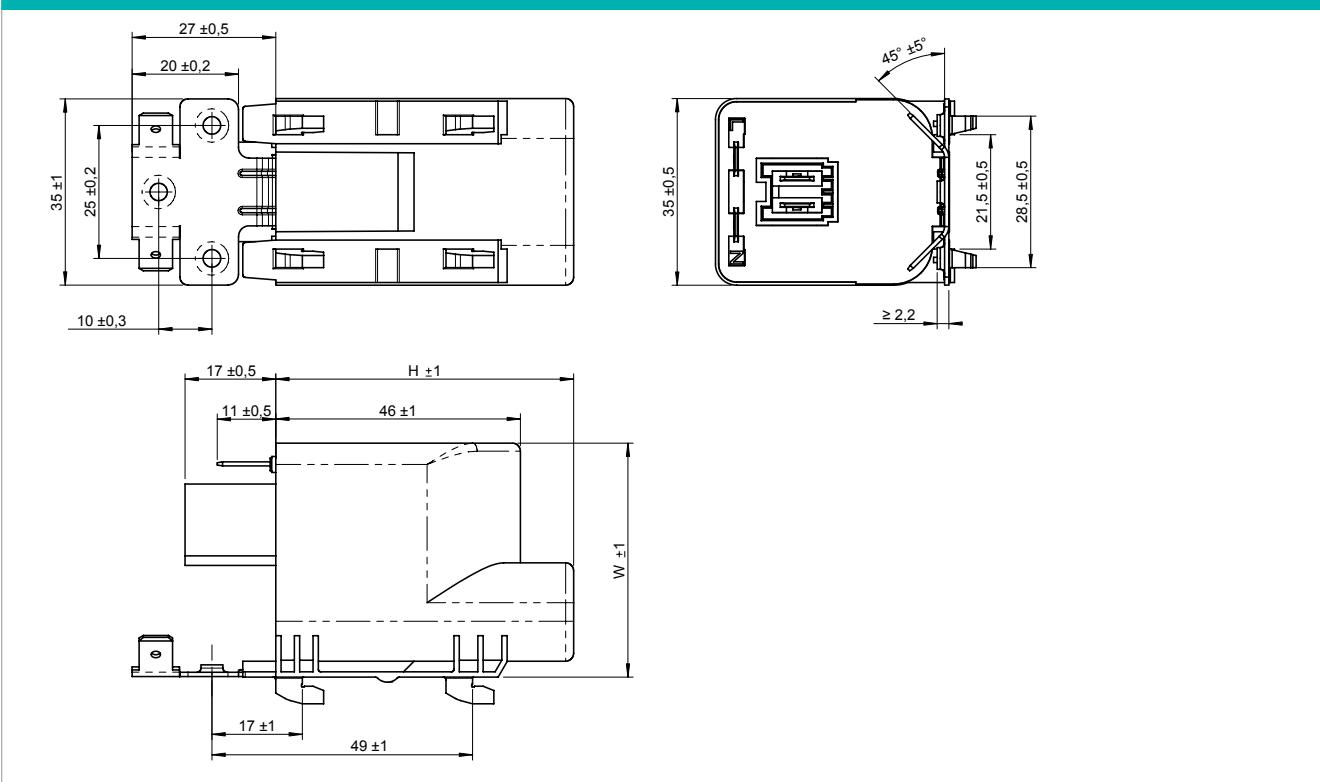
Casing: thermoplastic can, sealed with synthetical resin, flame retardant
