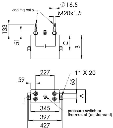
Picture 5 -KLS x200 Double Cooling Coils Capacitor
