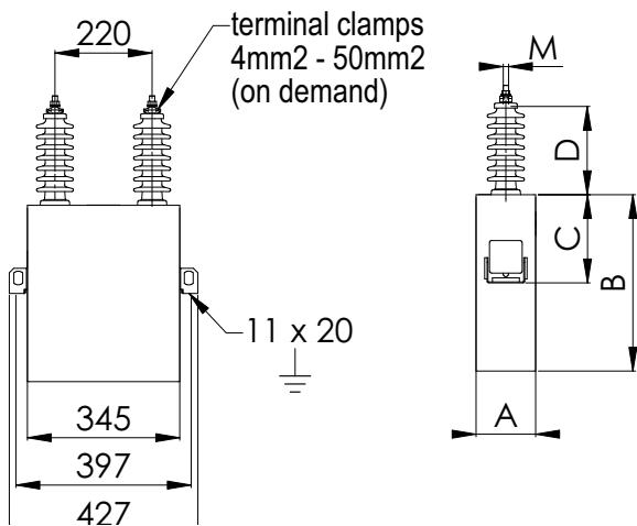
Picture 2: Single - bushing capacitor KLVxx0 (voltage on the container)
