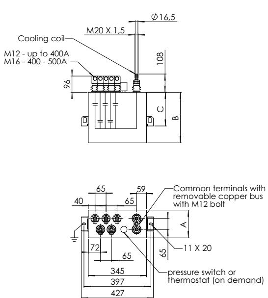
Picture 3 - KLS x2xx Single Cooling Coil Capacitor
