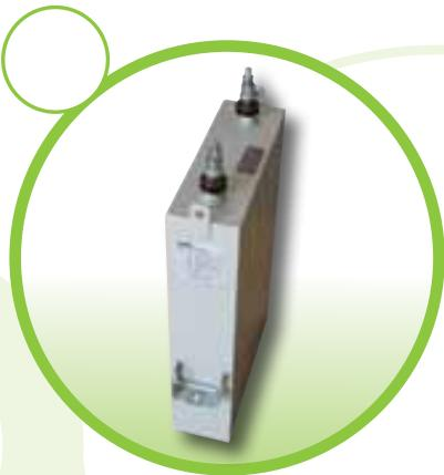
Advanced technology of low loss KLS capacitor units is based on construction of ALL-FILM capacitor sections and impregnation with environmentally compatible insulating oil (NON-PCB). Applications
