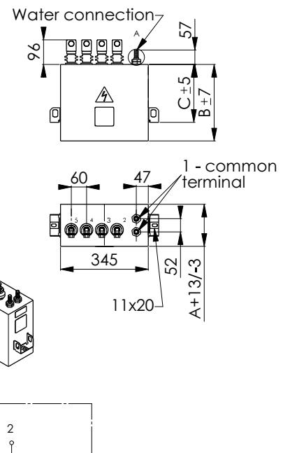
Picture 4 - KLS x400 Double Cooling Coils Capacitor - "dead"
