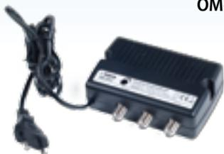
Antenna amplifier OM-2R/2 is suitable to amplify antennas, couplers or CATV signals through the coaxial cable. It enables signal distribution from antenna input to two outputs (two TV or radio sets). It is used only indoor; screws for fixing on wood are included.
